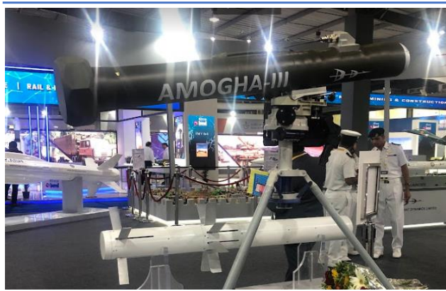
Exhibit 37: Amogha-III is a third generation fire-and-forget Anti-Tank Guided Missile – Bharat Dynamics
