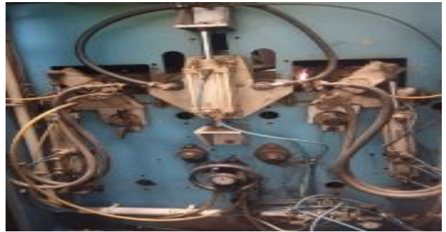
Figure 10: This machine features a flame that is used to remove excess defects from the fabric.
