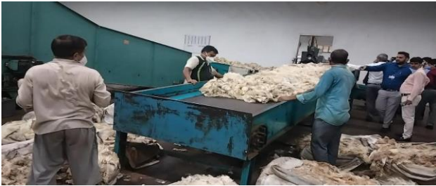
Figure 1: This machine is used to sort wool from animals like camels, rabbits, and sheep. The wool shown is Merino wool, which comes from Australia.
