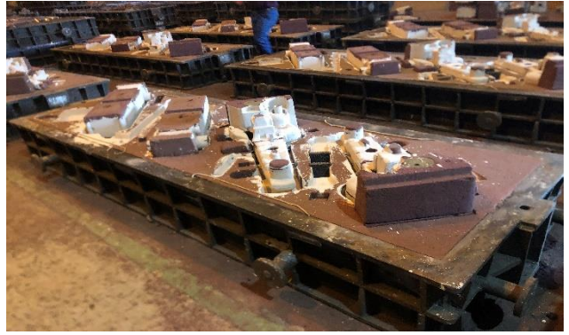
Exhibit 41: Molten alloy steel poured into mold to make components. The process take around 10 hours.
