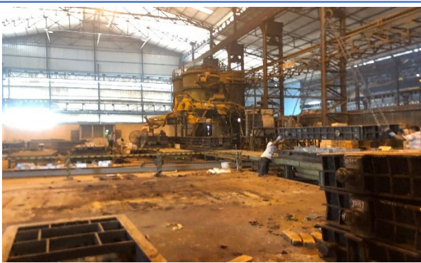
Exhibit 37: Sand Mixer is used to mix sand for molding process.
