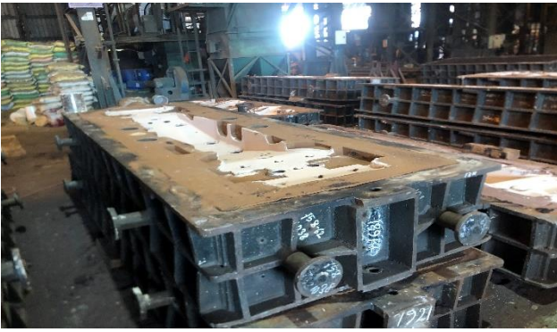
Exhibit 41: Molten alloy steel poured into mold to make components. The process take around 10 hours.
