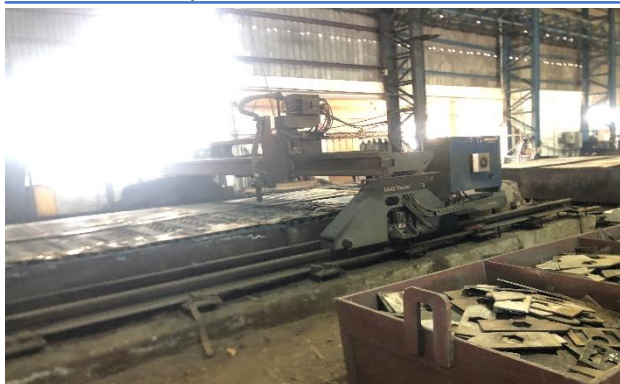
Exhibit 50: CNC Plasma cutting machine for making intermediate components.
