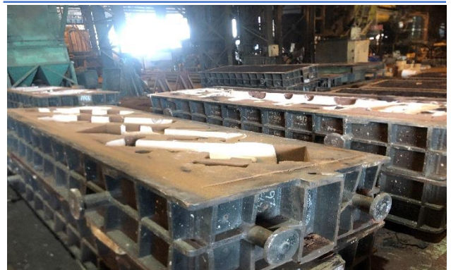
Exhibit 38: Molding made by Silica sand
