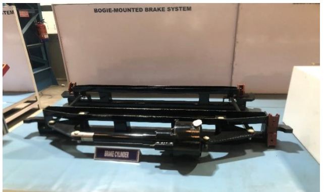
Exhibit 57: Bogie mounted for freight wagons.
